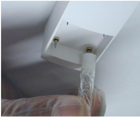
QuadBar cleaning. Be sure the alcohol does not flood the emitter point sockets
