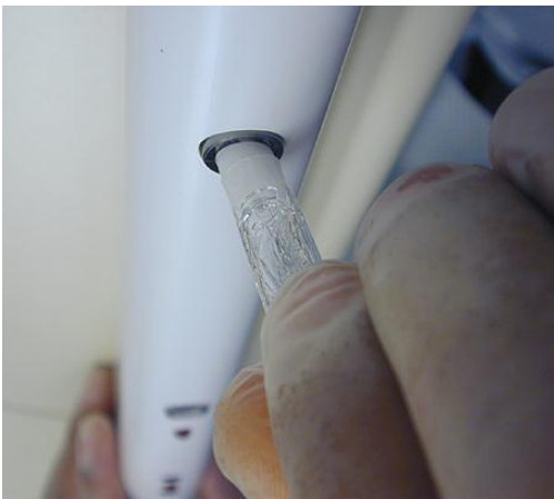
AeroBar cleaning. The brush will not fit all the way into the emitter nozzle. Ensure the brush swabs the tip of the emitter point
